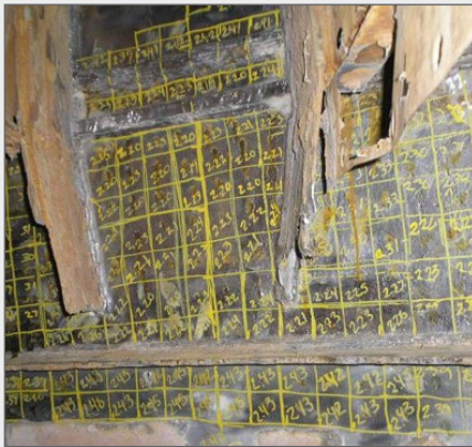
Thickness Mapping for Evaluation of Wall Loss Due to Corrosion
