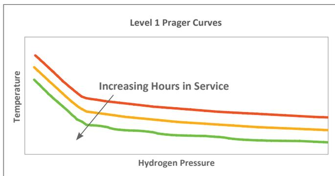
Failing a Level 1 FFS assessment is not the end of the story. Instead, a more sophisticated Level 2 FFS can be performed by running the Buckeye Model for HTHA assessment.
