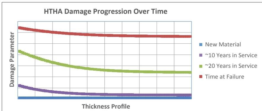
Damage prediction of a carbon steel heat exchanger operating at ~750°F at ~200 psia hydrogen
