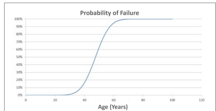
Our experts at E<sup>2</sup>G assess components using the Buckeye Model. Detailed information for equipment operating in HTHA environments is often limited. Statistical methods are used to characterize uncertainty, and probabilistic models are used to estimate the probability of failure over time.
